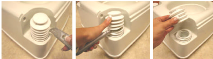
Cut half off the bellow with the knife and, take the bellow out.
