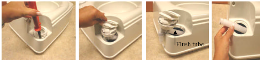
Note : Turn the water tank around when holding the bellow with the pincers. Take the bellow off the flush tube.
