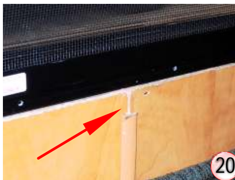
Bottom of window. T-section cut out the same height as the clamping.
