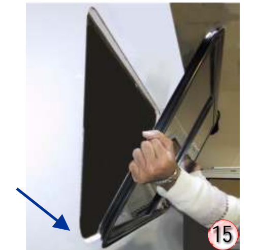
Position window in opening on the wall of the van where it is going to be installed. Do this from the outside of the van.
