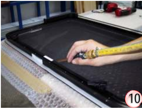
Clean window from aluminium swarf by blowing away with compressed air.
