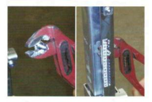
8 – Hold bolt in new hole position with vice grips and tighten nut with socket.
