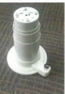
11 - Proceed to attach the table top slide mechanism to the leg. Position the table top slide mechanism on top of the table leg, lining up the four holes in the slide mechanism with the four screw holes in the table leg. Using the four screws you removed in step 2, fasten the table top slide mechanism to the table leg.
