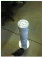
2 – Unscrew the four screws that are securing the plastic cover at the top of the table leg. And unscrew the two screws that are securing the plastic cover at the bottom of the leg.
