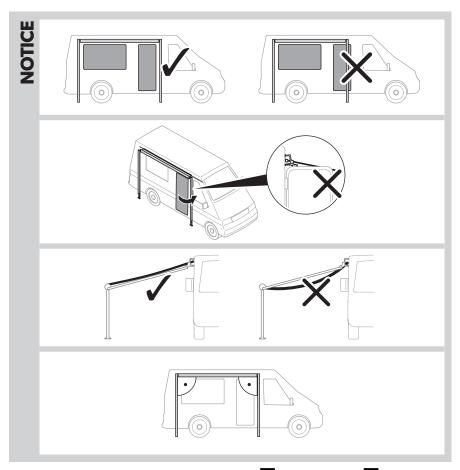
➤ Proceed as shown to install the awning (fig. 3 , page 10 to fig. 15 , page 17).
